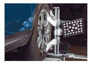
With a lightweight and durable design, AC700 clamps have the capacity to easily accommodate rims that range from 11"-22".
